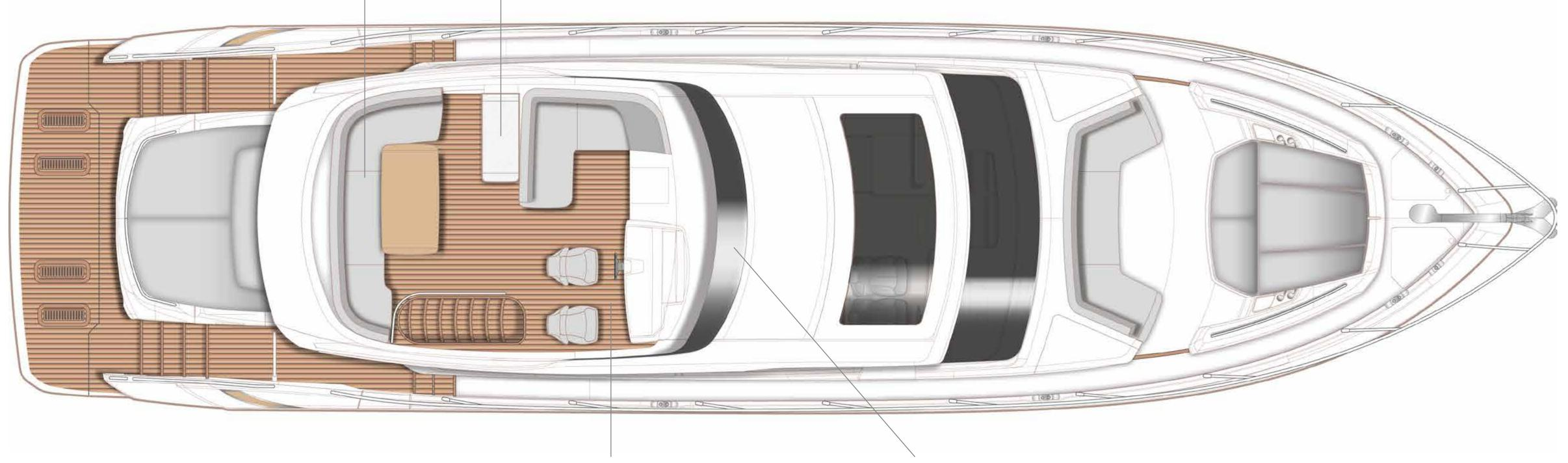
Dual station instruments and controls (see lower helm position on page 25); twin helm seats with fore and aft adjustment for helmsman, and adjustable steering wheel
