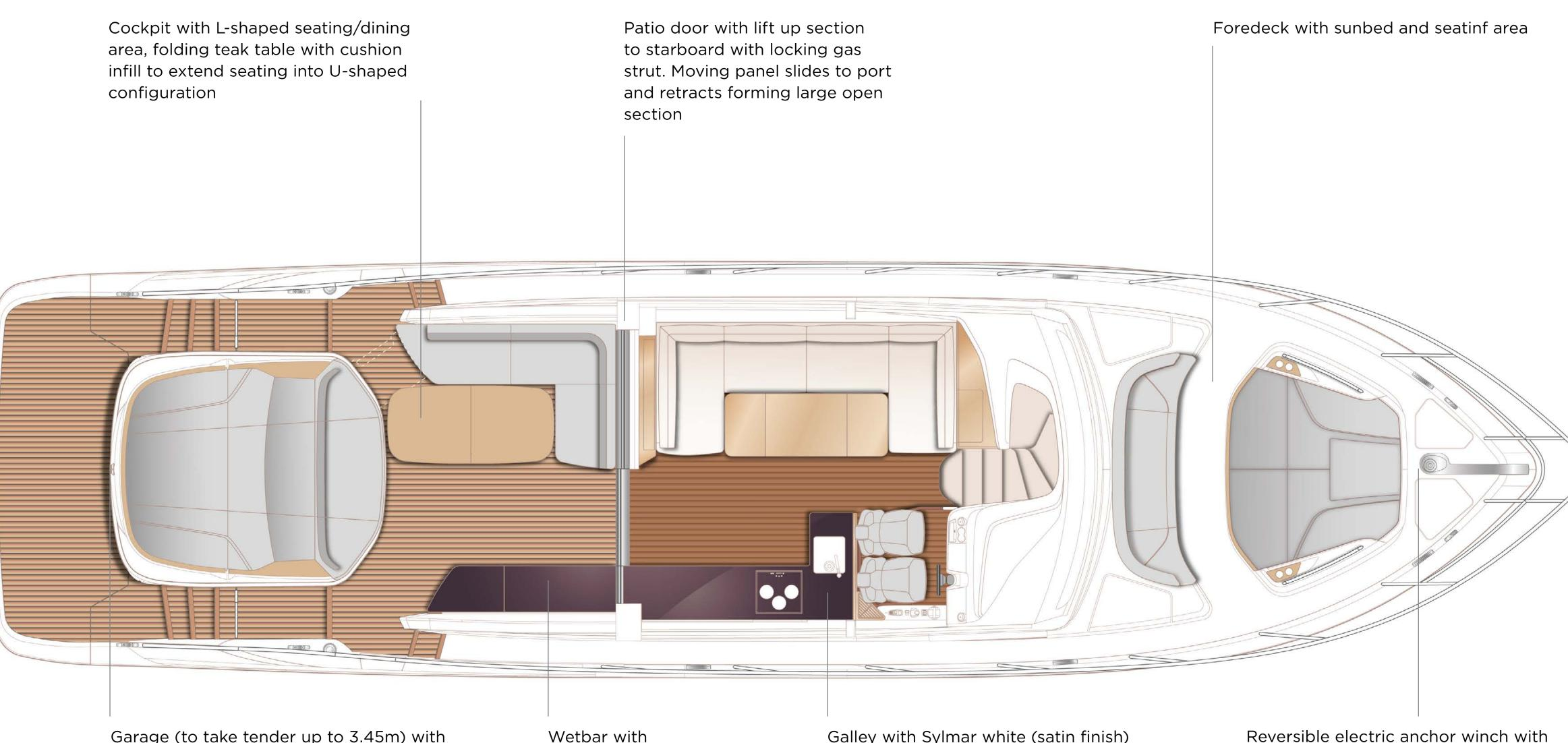
Garage (to take tender up to 3.45m) with electro-hydraulic door and tender launch system with electric winch; Electro-hydraulic raise/lower teak laid bathing platform (450Kg SWL); Retractable bathing ladder (manual) in side of hydraulic platform
