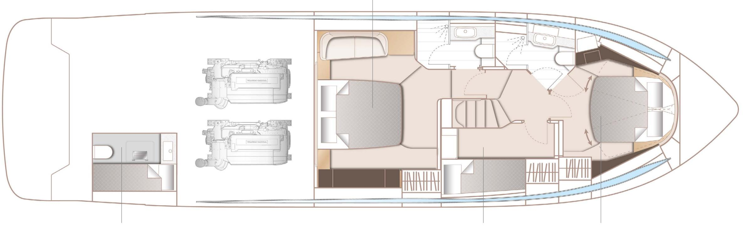
Optional Crew Cabin with single bed with storage below, storage locker, opening porthole, LED overhead lighting (24V), individual berth light, 220/240v outlet (1). non-slip safety flooring, mirror and washbasin with Solid Surface worktop
