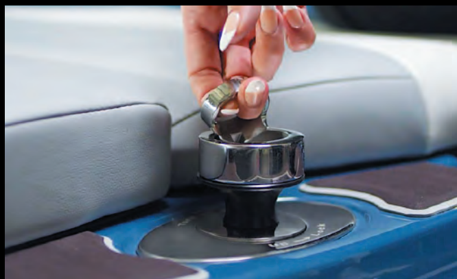
Pop-Up Ski Pylon: Seamlessly integrated, the pop-up ski pylon gives you even more watersports options and it's recessed when you don't need it.
