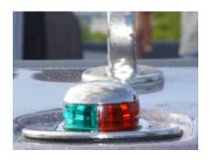
Bow lights are located at the front of the bow. On some models, it is two-colored—red and green and operated from a switch on the dash panel, while on other models there is a green light on the starboard side and a red light on the port side.
