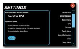
Touch ABOUT [UPDATE] to view the installed software version and instructions for how to install a software update here.
