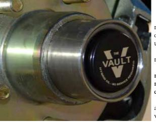
rear of the hub is sealed. The slight pressure inside the hub is needed to keep water out of the hub chamber when the hub is submerged underwater during loading and unloading.
