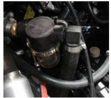
Raw water from the lake/river/sea is drawn into the boat to cool the engine and drive train. Even in closed cooling systems, it is necessary to circulate water in part of the system. To protect the system, a sea strainer is installed near the raw water intake and serves the purpose of keeping debris from entering the cooling system and causing eventual engine failure. As with any kind of strainer, it is necessary to regularly clean it so that water can flow unimpeded.
