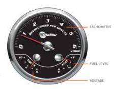
The lower right side of the gauge shows the approximate level of the fuel in the fuel tank. Note that movement of the boat can affect the reading, especially as fuel levels lower. Be certain to read the Fueling information in the Get Ready section of this Owner's Manual before operating the boat for important information
