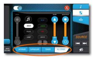
Backlighting Zones: The zone backlighting buttons, INTERIOR/CUPHOLDER/TOWER/ALL ZONES, allow each button to match the selected color and mode of that zone
