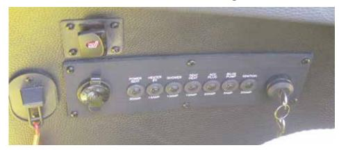
All major boat circuits are protected from shorting and overload by resettable circuit breakers. If a problem develops with one of the circuits, switch OFF the circuit and wait about one (1) minute. Then push the appropriate breaker button fully and switch on the circuit. If the circuit continues to trip, there is a problem somewhere in the system. Take your boat to an authorized Malibu dealer to locate and safely correct the issue.
