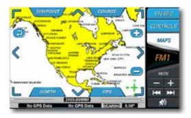
Touch anywhere on the map to activate the pop-up controls. Touch the six directional arrow buttons along the perimeter of the map window to position the cursor. Touch the RETURN button to return the cursor to the current location and the +/- buttons to zoom in or out.
