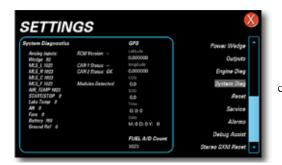
Touch SYSTEM DIAG to view on-screen system diagnostic information concerning bat sensors and GPS signal.
