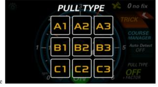
get back to the set speed. The lower the letter (A being the lowest) the longer it will take for the engine to respond to the speed drop. The higher the letter (C being the highest) the faster the engine will respond to the speed drop.
