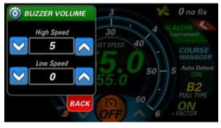
The buzzer volume adjustment compensates for increased engine noise. As the boat speed increases, and therefore the noises from the engine increase, the volume of the buzzer will increase proportionately to the boat's speed between 0 and 25 mph (40.2 km/h). No further increase occurs at speeds above 25 mph (40.2 km/h). The buzzer emits a sound when the set speed is reached and when reaching the buoys at a course. Select Buzzer Volume, and the following appears:
