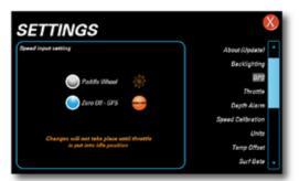
Touch GPS to change the speed signal source from ZeroOff to PADDLEWHEEL. The default is ZeroOff. The boat must be at idle throttle when changing this setting.
