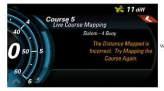
Press the End Gate button when crossing the final gate. If the mapping was unsuccessful, this screen will appear.
