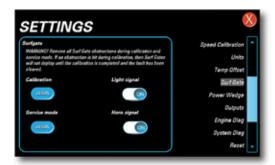
Touch SURF GATE to calibrate, service or toggle the audible and visual indicators for Surf Gate, switching on or off. The SERVICE and CALIBRATE can be done only at idle. Service drives both surf actuators out and then back in. Calibration will pulse both actuators in and continue to pulse them in until the boat is stopped.
